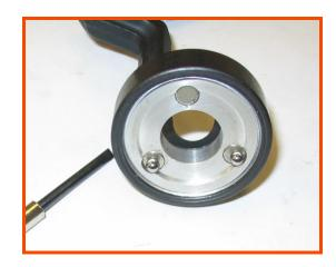
3a. Take the Magnetic Lath Nosepiece – align it with the rib in the nose casting and place the threaded end in the depth adjustment dial.
