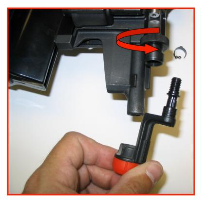
\* Use magnets to hold ball bearings. Until replacing them.
