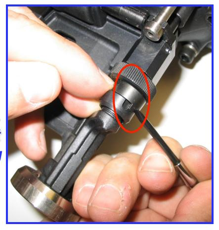
6. Finally, Rotate Depth Adjusting Knob, clicking detent noise should be heard as you turn either clockwise or counter clockwise.
