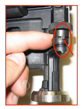
5A. Carefully, replace Snap Ring over Ball bearings – the ball bearings easily fall out. Possibly use a dab of petroleum grease to hold them in.
